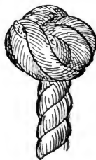
FIG. 123.—Double wall (complete).
